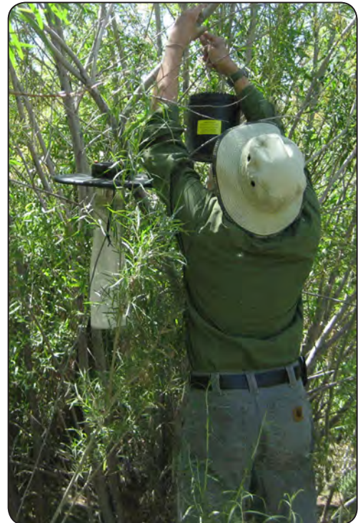
A staff member hangs a Encephalitis Vector Surveillance (EVS) trap near a known mosquito breeding source in Mesquite, Nev.
